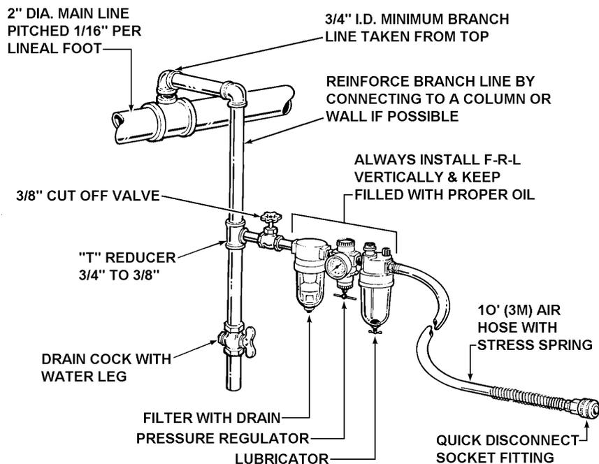
Filter and lubricator bowls are made of polycarbonate material. Do not install where bowls may be exposed to materials incompatible with polycarbonate. Certain oils, solvents, and chemicals or their fumes can weaken these bowls and possibly cause them to burst. Clean only with warm water. A cut-off valve placed ahead of the filter will be useful when cleaning the filter or replenishing the lubricator.
